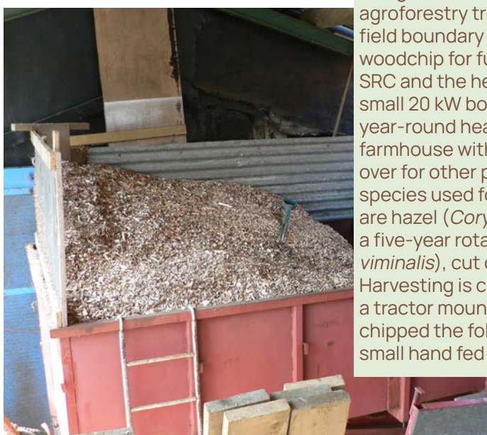
From field to boiler. Willow harvested, dried and chipped to feed into a woodchip boiler that heats the farmhouse.
